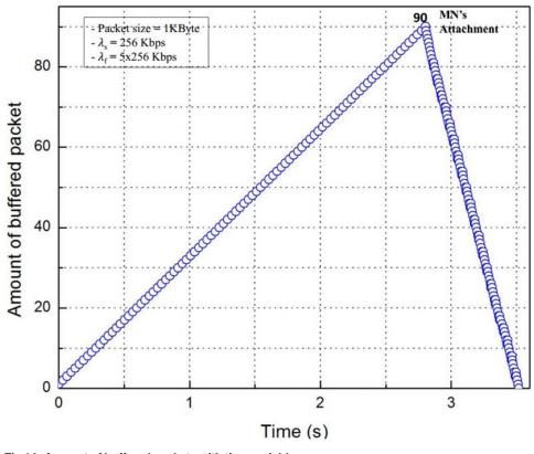
Fig 14. Amount of buffered packets with time variable.
