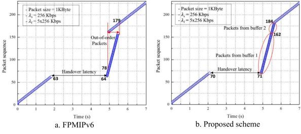
Fig 11. Packet flow with  $\lambda_s = 256$  Kbps,  $\lambda_f = 5\lambda_s$ . (a) FPMIPv6, (b) Proposed scheme.
