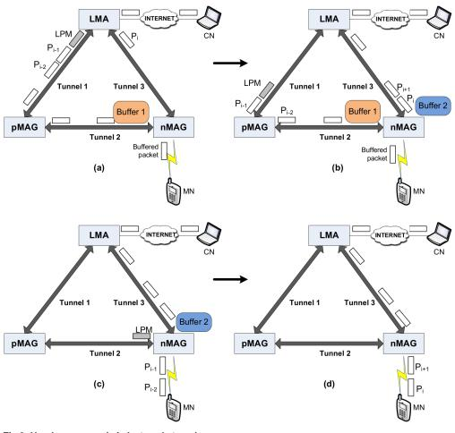
Fig 3. Handover scenario in last packet marker.
