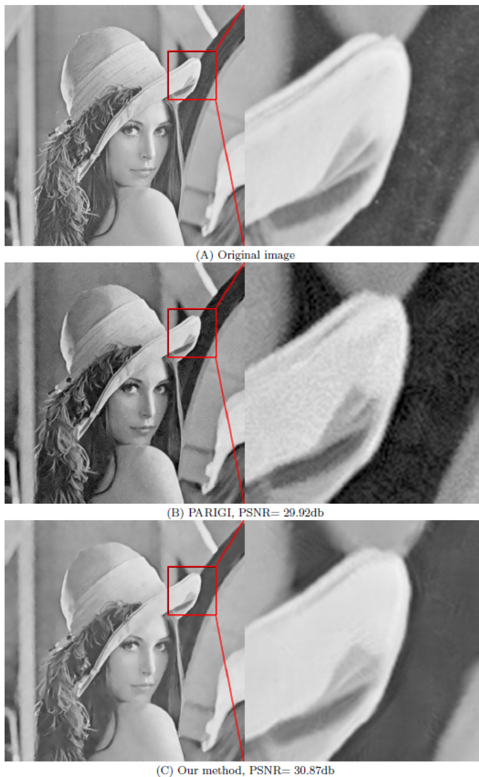
Fig 4. Comparison between PARIGI and our method (OWMF) for image “Lena” contaminated by Gaussian noise with \sigma = 20 and impulse noise with p = 20\% . (A) the original image and its part; (B) the image restored by PARIGI and its part; (C) denoised image by our method and its part.
