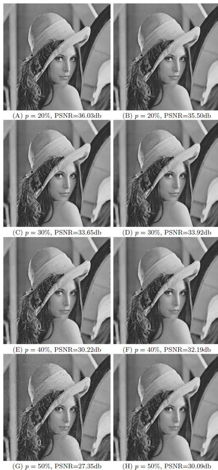
Fig 2. Restored images contaminated by pure impulse noise using our method (OWMF) with different sizes of the detection window \Omega_{\sigma, \sigma}^0 . The first column corresponds to images restored with size 3 \times 3 of the
