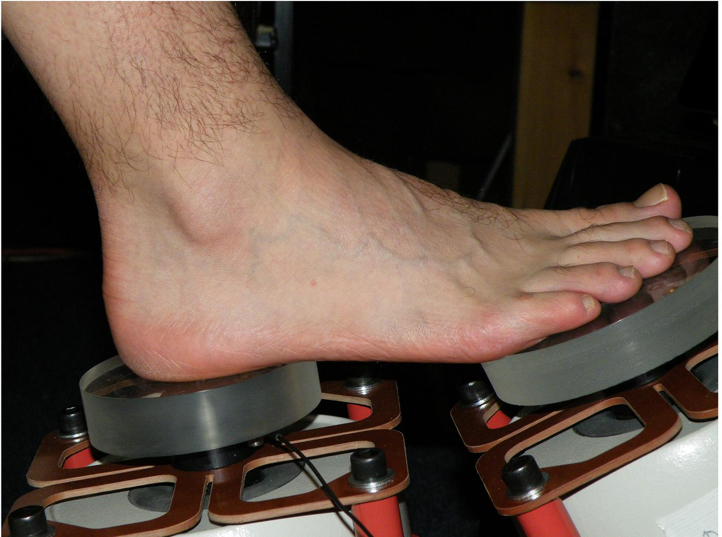
**Fig 3. Electrodynamic shakers and contactor discs used to present vibration to the forefoot or the heel.**
