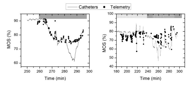
Figure 8. Mixed oxygen supply (MOS) measured by the telemetry sensor (black dots) and the reference equipment (grey line) for both studies (1: left, & 2: right). doi:10.1371/journal.pone.0102396.g008
