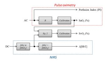
**Figure 3. Flow chart of the signal processing.** This was employed to compute the oxygen saturation at the arterial and venous side along with perfusion changes from the measured AC and DC signals. doi:10.1371/journal.pone.0102396.g003
