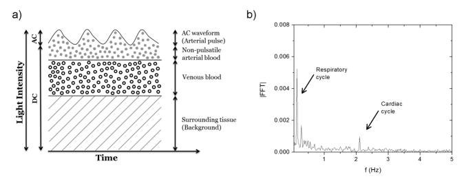
**Figure 2. Typical PPG signal.** a- Schematic of the collected reflectance signal (Note that the various signal components are not drawn to scale to allow easy visualization). b- Spectrum of the reflectance signal collected with our sensor prior to amplification and with the DC signal omitted. doi:10.1371/journal.pone.0102396.g002
