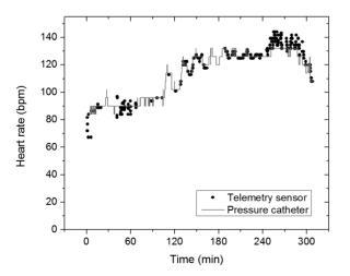
**Figure 4. Heart rate measurements.** Data from the arterial pressure catheter (grey) and the telemetry sensor (black). doi:10.1371/journal.pone.0102396.g004
