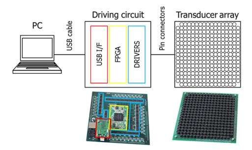
**Figure 2.** Phased array modules. (Left) The phased array modules are operated by a computer via USB. (Middle) Each driving circuit board consists of three components; USB I/F, FPGA, and Driver ICs. (Right) Each phased array module has 285 ultrasonic transducers. doi:10.1371/journal.pone.0097590.g002
