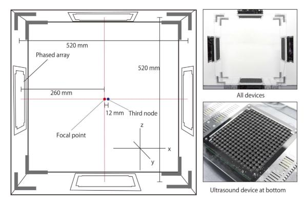
**Figure 3. Illustration and photograph of system setup.** The size of system is 520 mm(height) $\times$ 520 mm(width) $\times$ 250 mm(depth). The focal point is set in the center of workspace. The labels of axis are shown in the figure: x-axis and z-axis are parallel to the device plane and y-axis is vertical to the device plane. We inserted the particles at the third node of beams that is parallel to x-axis in the stability experiments. doi:10.1371/journal.pone.0097590.g003
