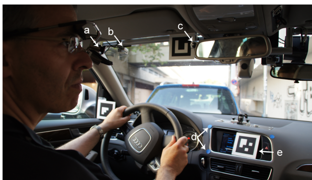
Figure 1. (a) A participant, wearing the mobile eye-tracking head unit; (b) First camera recording the road scene during the drive; (c) Second camera recording the driver during the drive; (d) Calibration points; (e) Scene marker used for calibration. The subject has given written informed consent, as outlined in the PLOS consent form, to publication of their photograph.
