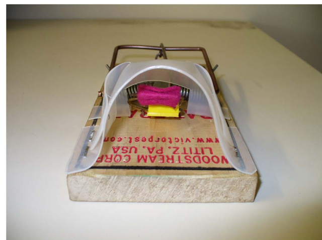
Figure 4. Set trap showing position of the new copper rod and felt trigger. doi:10.1371/journal.pone.0086760.g004
