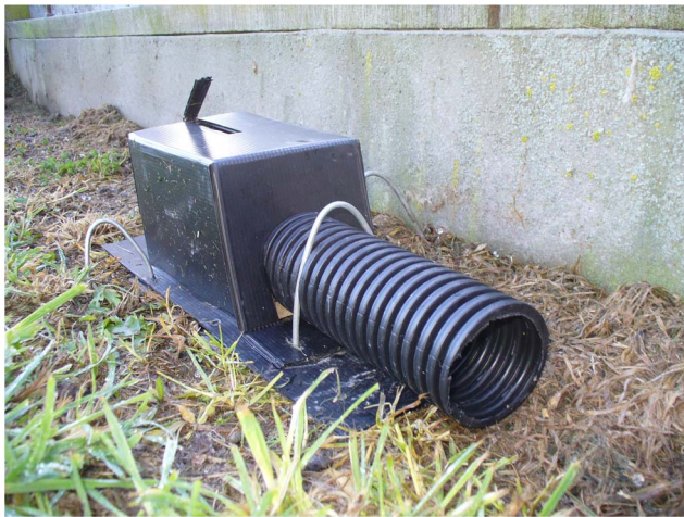
Figure 5. Trap cover for horizontally set Victor professional rat trap. Note slot cut in top of tunnel to allow trigger wire to freely extend upwards when trap is triggered. doi:10.1371/journal.pone.0086760.g005
