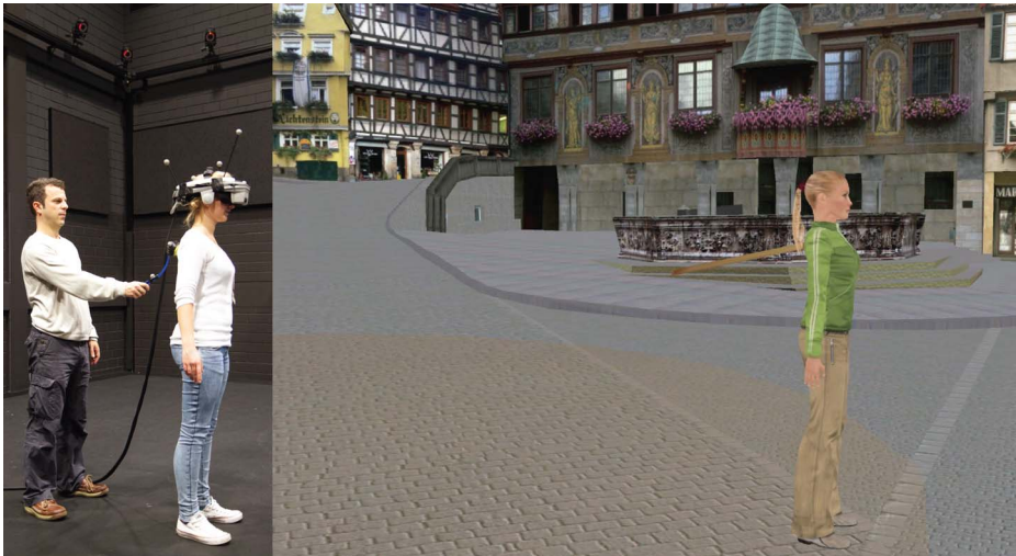
Figure 1. The experimental setup. The experimenter strokes the physical back of a female participant with a motion-tracked stick while she watches, on a head-mounted display, a virtual body (side view) from behind at a distance of 5 meters being synchronously stroked with a virtual stick. The subjects on the photograph have given written informed consent, as outlined in the PLOS consent form, to publication of the photograph. doi:10.1371/journal.pone.0083840.g001
