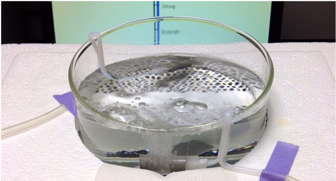
Figure 3. Beaker that contained the stimulus solutions. Inserted into the beaker were two HPLC filters through which air flowed to create bubbles. Subjects sampled the solutions by inserting the tip of their tongue over the near HPLC filter. Under the control of a solenoid valve, bubbles could be presented under the tongue (as shown, or away from the tongue (by directing air to the further HPLC filter). In the background, a computer monitor is visible (subjects could see it clearly). On the monitor is an LMS scale. Subjects continuously tracked bite intensity by moving a mouse that controlled the height of blue bar next to the LMS. doi:10.1371/journal.pone.0071488.g003
