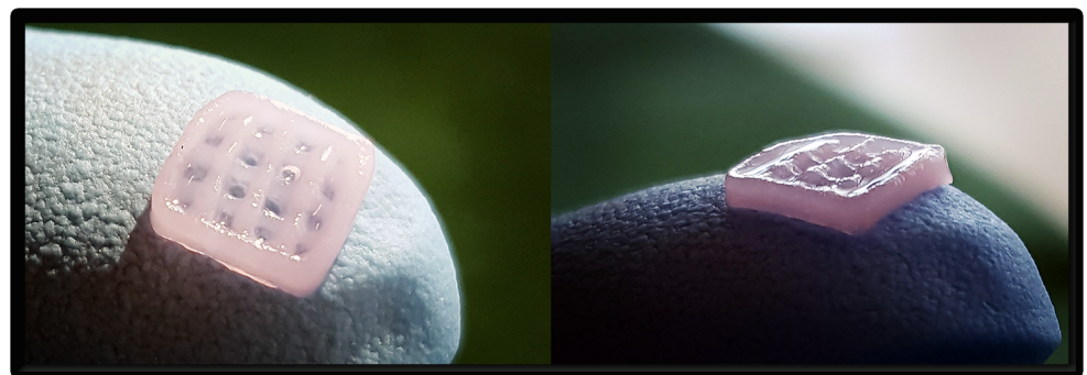
Fig 1. 3D-bioprinted grid. Example of a cell-containing grid ( 5 \times 5 \times 1.2 mm) with a line spacing of 1.5 mm in three layers.
