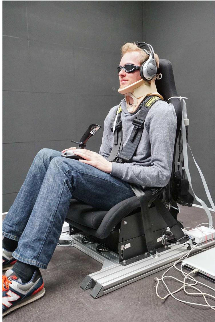
**Fig 1. Experimental setup.** The figure shows the platform seat mounted on top of the motion platform, with rails that allowed for small position adjustments prior to the experiment to ensure head-centred rotation (see text). Participants were blindfolded and secured with seat belts. White noise played through the headphones and ear plugs masked auditory cues from the simulator, goggles prevented visual motion cues and a neck brace helped maintaining the head stable.
