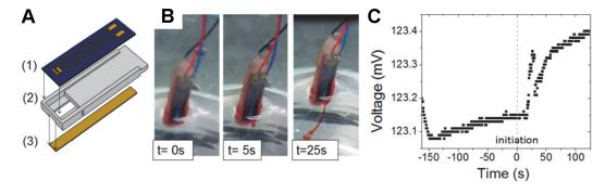
**Figure 4. Drug delivery device activation.** A) Assembly of the drug delivery unit B) vasopressin ejection over 25 s of applied voltage C) increase in biosensor voltage due to drug delivery. The vertical dotted line indicates when the potential was applied (at t = 0 s) and the a sustained spike in voltage occurs after 25 s. doi:10.1371/journal.pone.0089903.g004
