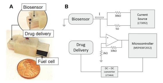
Figure 1. hemoAID device and schematic of electrical connections. A) Integrated device consisting of a biosensor, drug delivery and fuel cell unit B) schematic of the electrical connections between the different components of the hemoAID. doi:10.1371/journal.pone.0089903.q001
