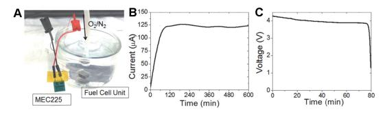
**Figure 5. Power unit characterization.** A) Power unit consisting of a 1 cm<sup>3</sup> fuel cell unit in 5 mmol glucose solution at 8% O<sub>2</sub> saturation and an external rechargeable battery B) chronoamperometric response of the fuel cell unit at 0.1 V in 0.01 M PBS solution and 5 mmol/L glucose solution over a period of 10 h C) discharge profile for the rechargeable battery at an operating current of 100  $\mu$ A. doi:10.1371/journal.pone.0089903.g005
