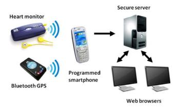
Figure 2. Components of remote monitoring system. doi:10.1371/journal.pone.0014669.q002
