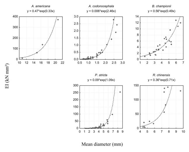
**Figure 9. Bending rigidity.** Bending rigidity (*EI*) as a function of root mean diameter for each species where data were sufficient for statistical analyses. Mean root diameter is the mean of depth and width diameters for each root. Note that scales differ between graphs for easier viewing. doi:10.1371/journal.pone.0095876.g009
