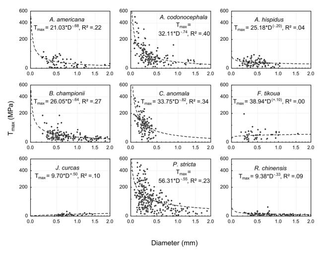
Figure 7. Tensile stress at failure. Tensile stress at failure ( $T_{max}$ ) for root diameters from 0 to 2 mm. Logarithmic scales. Fitting curves:  $T_{max} = \alpha * D^{-\beta}$ , equations are presented on the graphs with the determination coefficient ( $R^2$ ), parameters in brackets are not significant. doi:10.1371/journal.pone.0095876.g007
