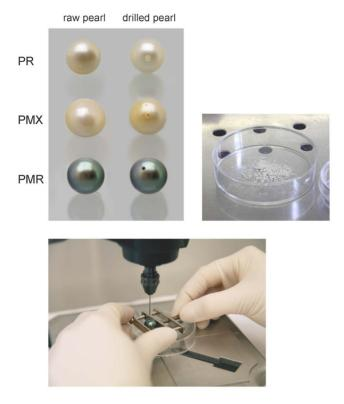
**Figure 5. Examples of pearls of** *Pinctada margaritifera, P. maxima* **and** *P. radiata* **used in this study before and after micro-drilling.** We used a drill head attached to a Dremel Workstation to produce pearl powder used for DNA extraction. Recovered pearl powder (nacre and organic material) can be seen in the Petri dish. *P. margaritifera* (PMR), *P. maxima* (PMX) and *P. radiata* (PR). doi:10.1371/journal.pone.0075606.q005
