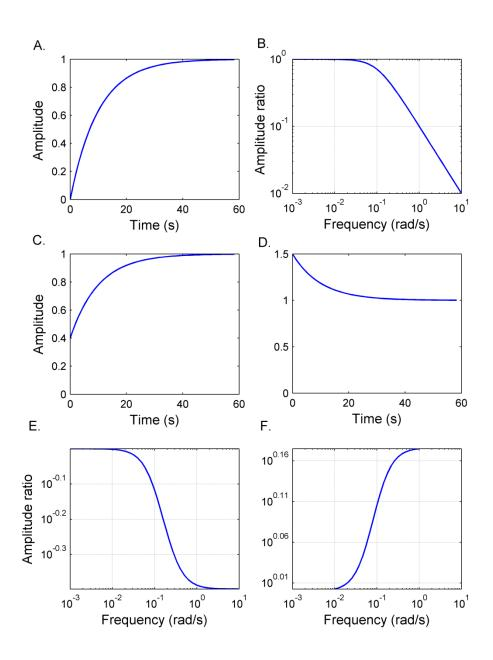
Figure S18. Time and frequency domain responses of first order lag and lead-lag systems. (A) Step, and (B) frequency responses of a first order lag system. In (B), breakpoint frequency is equal to  $1/\tau_p = 0.1$  rad/s. Unit step responses of lead-lag processes with (C)  $\tau_z/\tau_p$  < 1, and (D)  $\tau_z/\tau_p > 1$ . Magnitude Bode plots of lead-lag processes with (E)  $\tau_z/\tau_p < 1$ , and (F)  $\tau_z/\tau_p > 1$ .
