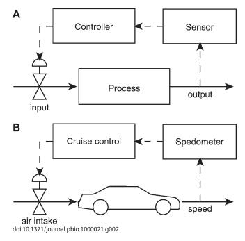
Figure 2. Examples of Control Loops
