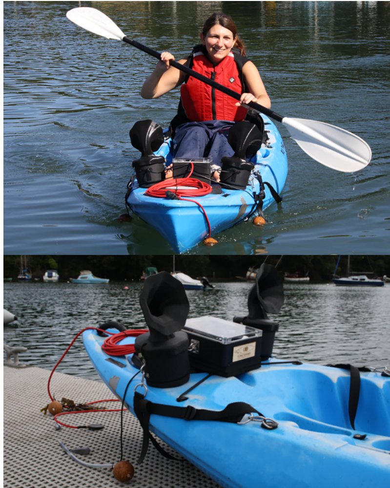
Fig 2. The Sonic Kayak system.
